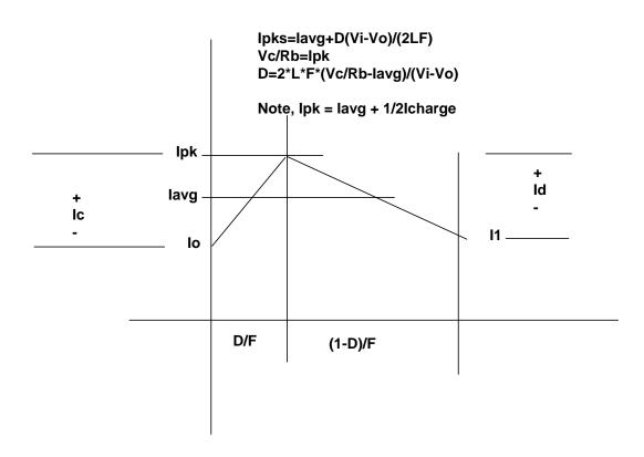
Where Vc = Control Voltage Rb = Burden (Sense) Resistor D=Duty Ratio L= Inductance of the switched inductor F=Switching Frequency
