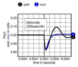
Figure pid. Test results show the PID waveform ringing at the L-C resonant frequency.
