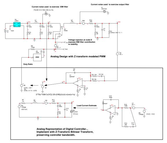
**Figure 2**, An analog model of the proposed DSP controller, see www.intusoft.com/DSP/Drawings/FwdTest.dwg, page 1.
