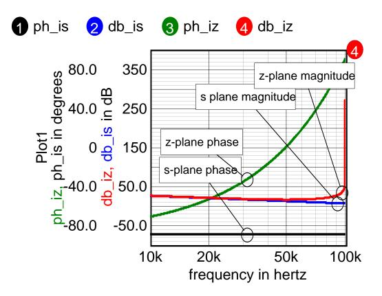
Figure z2, Z Transform of an integrator compared with continuous time integration
