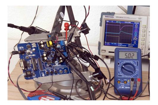
The test data in Figure pid shows how the 2 control loops respond to a 1 amp load step
