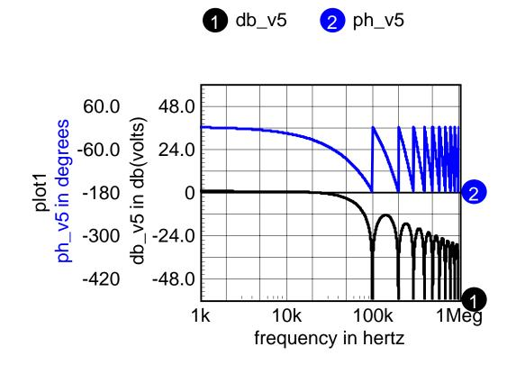
Figure z6 Zero order hold nulls signals at harmonics of the sampling frequency
