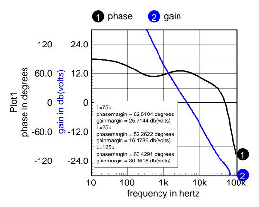
Figure 5, Outer control loop cut at V8
