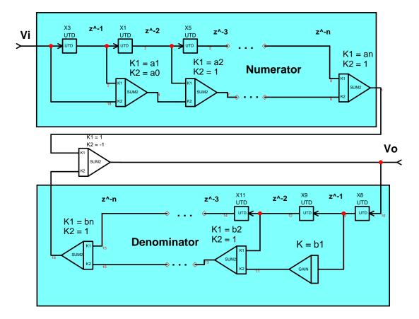
Figure z1, Direct Programming Method
