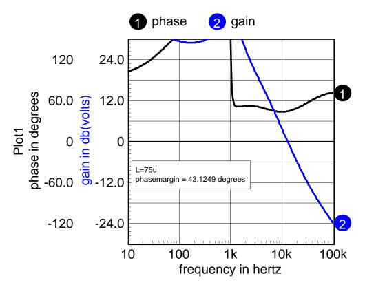
Figure 6, Plant matching loop cut at V7
