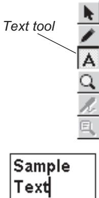
Text objects may be inserted directly on the schematic either from the Text Object in the Parts menu, or using the Text tool in the Tool Palette. Bring a schematic to view.
