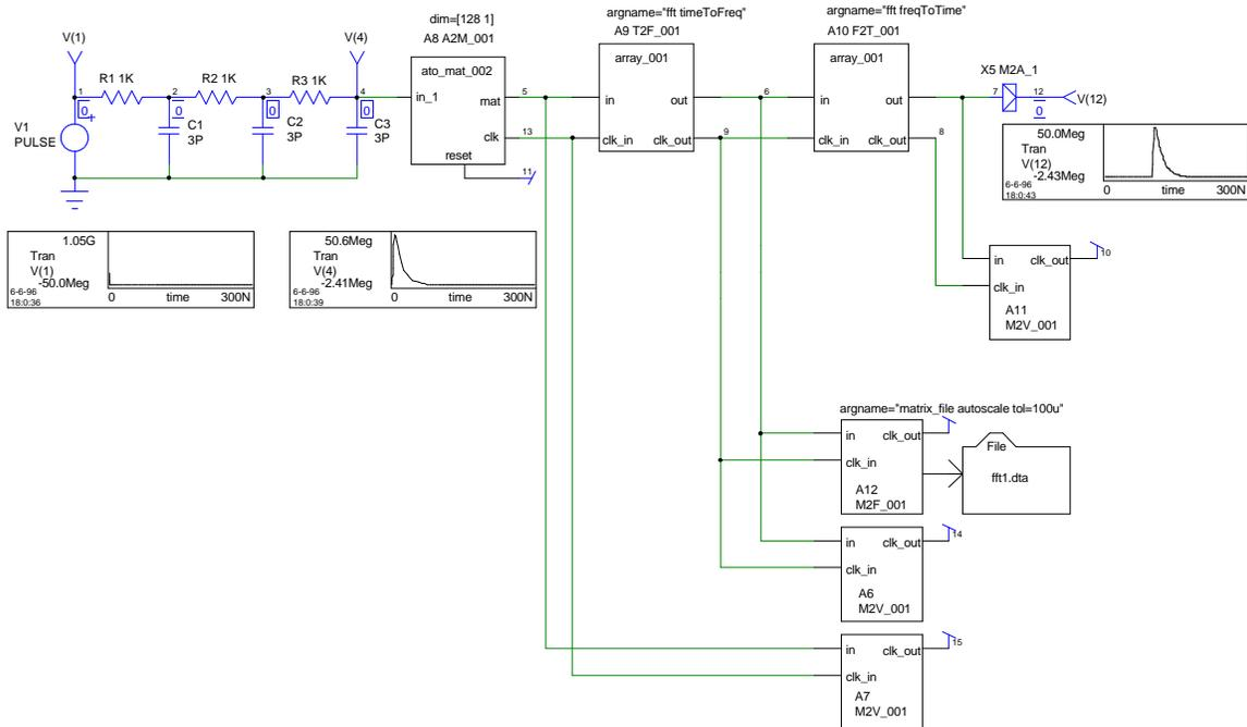
From the schematic we can see that an analog signal is converted to an array matrix, A8 A2M\_001, that is then sent to a Sink mode, A7 M2V\_001 (Bottom), controlled by the following model statement.
