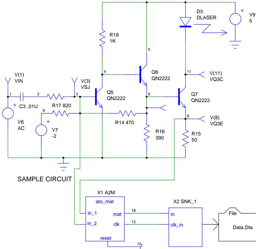
The portion of the schematic that is of interest in this example consists of the A2M, Analog-to-Matrix model and the SNK\_1, Sink Array model. These are X1 and X2 respectively.
