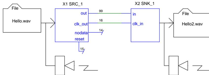
This circuit is comprised of two Array code models, a source (SRC\_1) and a sink (SNK\_1). The Source Array model reads input from a Microsoft .WAV file. The information from this .WAV file is sent directly to a Sink Array model that plays the .WAV file read by the source.
