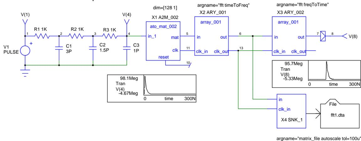
In this example we find two new Array elements, X2 and X3, performing an FFT and an IFFT respectively. The remaining elements have been discussed in other examples.
