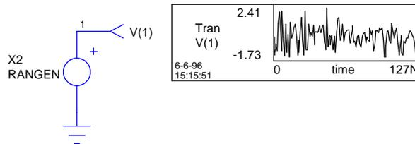
The circuit consists of one subcircuit that contains an Array Source model and an Matrix\_to\_analog bridge.
