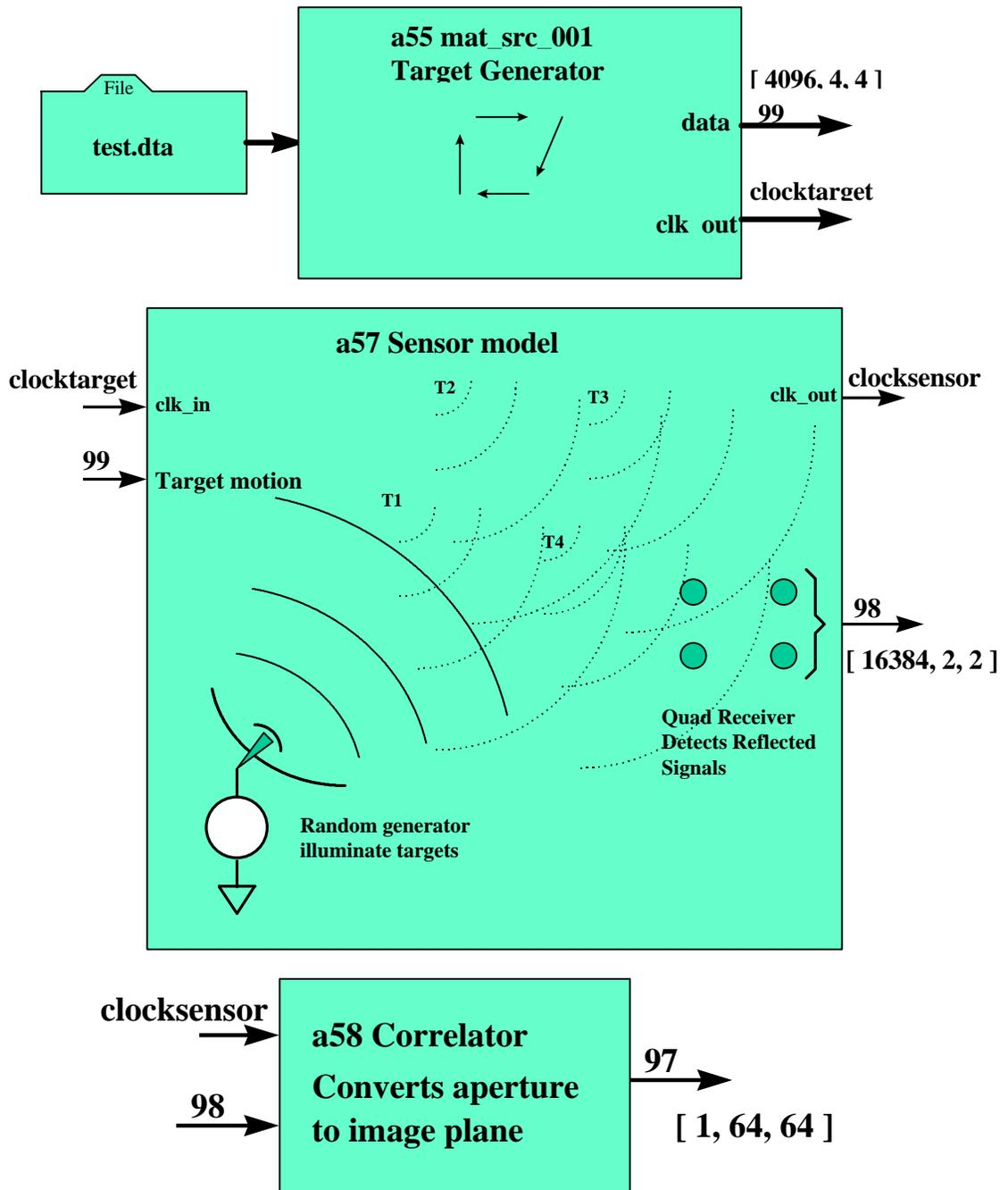
The return signals are detected using a quad sensor. The four time varying target signals, T1, T2, T3, and T4, can be thought of as samples at the aperture of a large lens. It may then be possible to map these signals to the focal plane and image the objects. To do this the way a camera works, one would perform a 2 dimensional Fourier transform, described in literature as a Fresnel equation.
