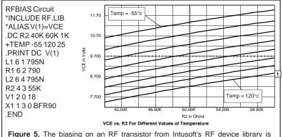
investigated by sweeping a resistor, R2, over a temperature range of -55°c to 120°c.
