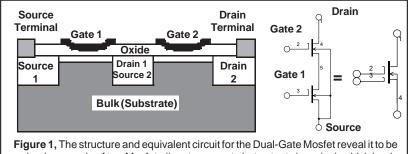
a simple cascode of two Mosfets (inputs separate but outputs in series), which leads to the resulting IsSPICE subcircuit configuration.
