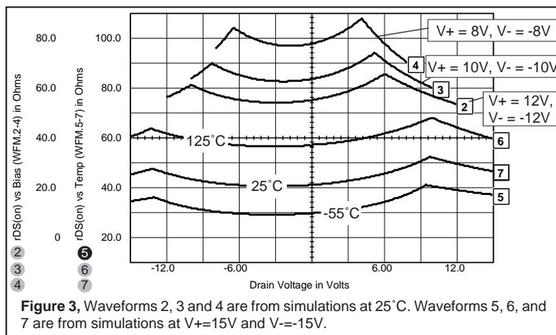
**Figure 3**, Waveforms 2, 3 and 4 are from simulations at 25°C. Waveforms 5, 6, and 7 are from simulations at V+=15V and V-=-15V.
