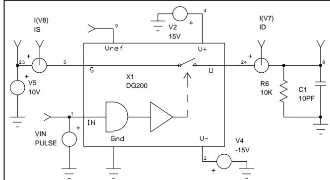
**Figure 2**, Test circuit for the DG200 CMOS analog switch (Siliconix). Setup shown is for the measurement of the delay, rise, fall, and switching transients.
