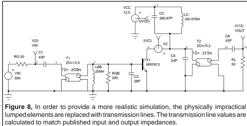
**Figure 8**, In order to provide a more realistic simulation, the physically impractical lumped elements are replaced with transmission lines. The transmission line values are calculated to match published input and output impedances.
