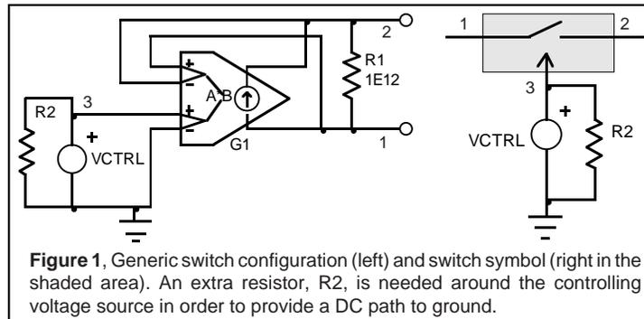
**Figure 1,** Generic switch configuration (left) and switch symbol (right in the shaded area). An extra resistor, R2, is needed around the controlling voltage source in order to provide a DC path to ground.
