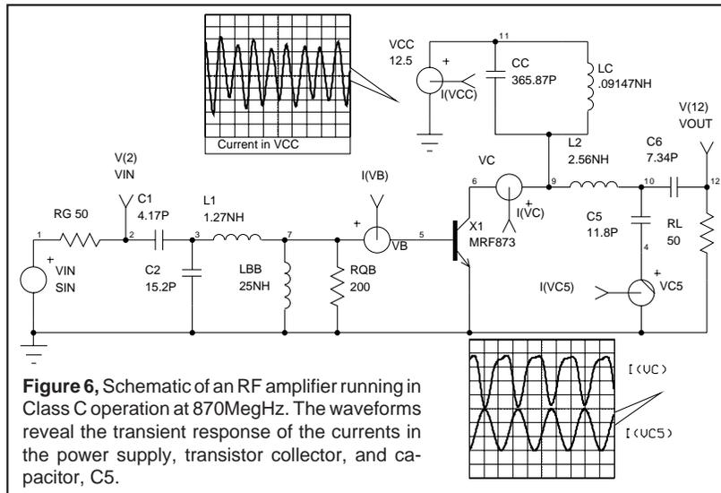
**Figure 6,** Schematic of an RF amplifier running in Class C operation at 870MegHz. The waveforms reveal the transient response of the currents in the power supply, transistor collector, and capacitor, C5.
