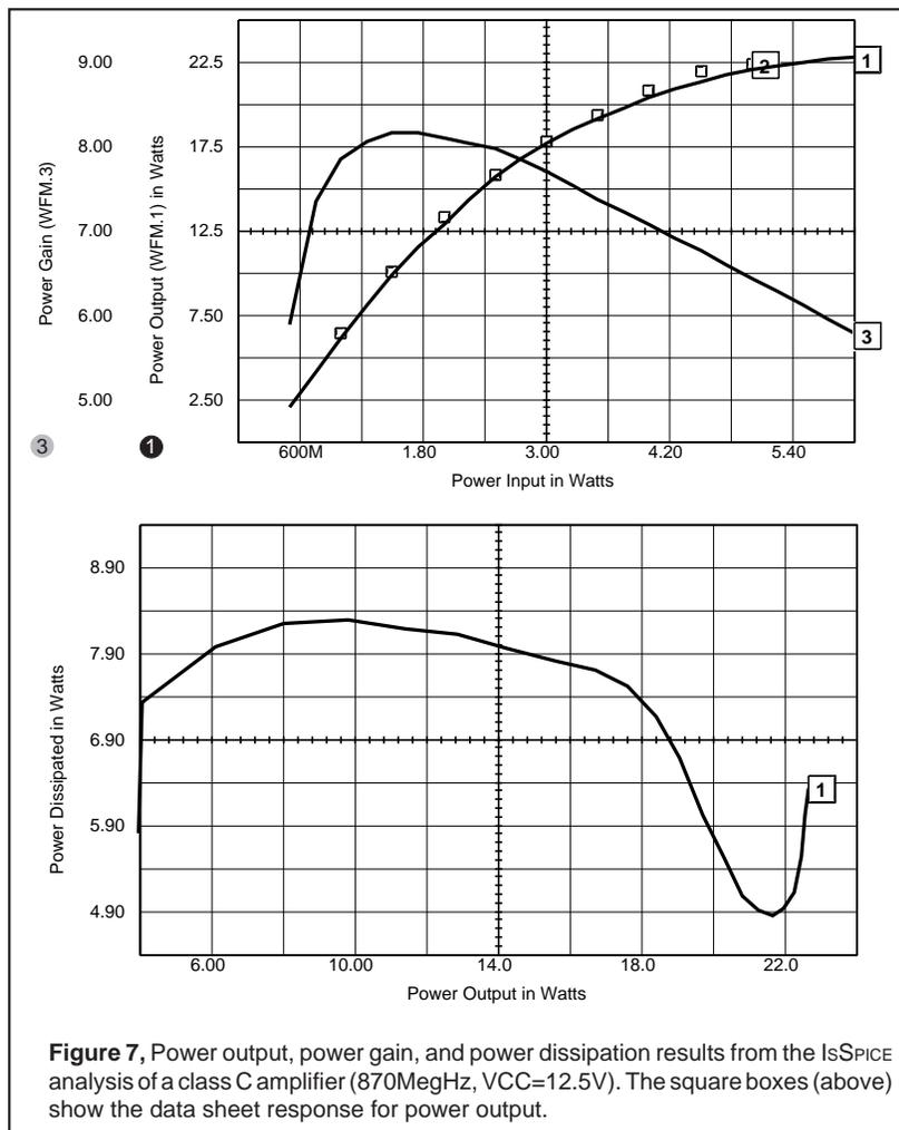
**Figure 7**, Power output, power gain, and power dissipation results from the IsSPICE analysis of a class C amplifier (870MegHz,  $V_{CC}=12.5V$ ). The square boxes (above) show the data sheet response for power output.
