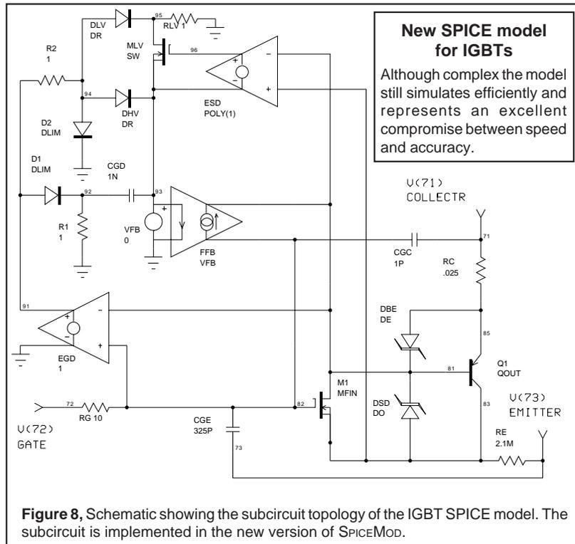
**Figure 8,** Schematic showing the subcircuit topology of the IGBT SPICE model. The subcircuit is implemented in the new version of SPICEMOD.
