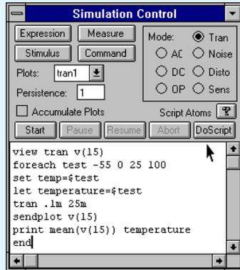
Figure 13, Opto-Isolator test circuit using the H-P CNR200 temperature insensitive isolation amplifier. The ICL script is run interactively from the IsSpice4 Simulation Control dialog.
