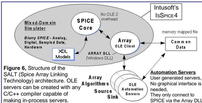
**Figure 6,** Structure of the SALT (Spice Array Linking Technology) architecture. OLE servers can be created with any C/C++ compiler capable of making in-process servers.
