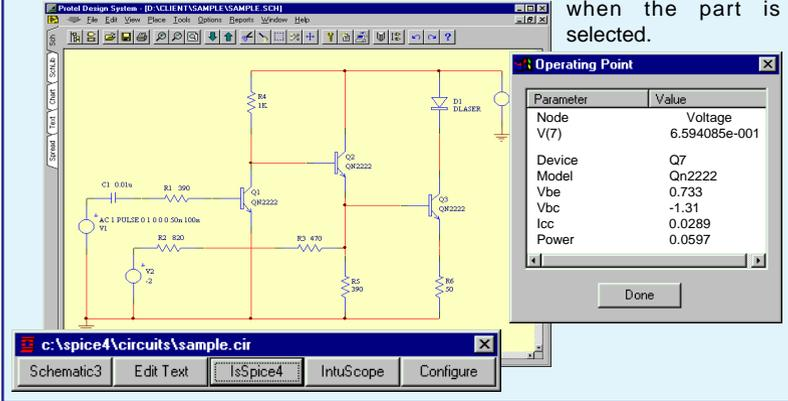
IsSpice4 is run by either creating a SPICE netlist or by selecting the "Run IsSpice4" menu function, depending on your schematic. When a simulation is run, the **ICAP™** Toolbar appears and IsSpice4 displays the simulated waveforms in real time (Figure 1). The communication is outlined in Figure 3.
