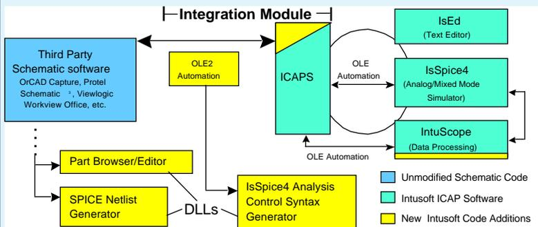
Several DLLs that enhance the schematic's ability to access SPICE attributes and other advanced simulation features are hooked into the schematic transparently using OLE technology.
