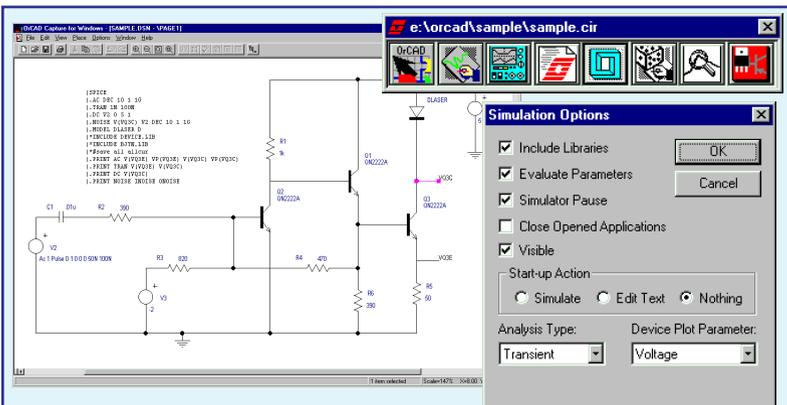
**Figure 2, The ICAP™ Toolbar** (top right) is customized for each schematic entry package (Capture shown above). It provides schematic users with easy access to model editing, SPICE simulation, cross-probing options, and real time waveform processing. Special menu functions have also been added to ease various simulation tasks (right).
