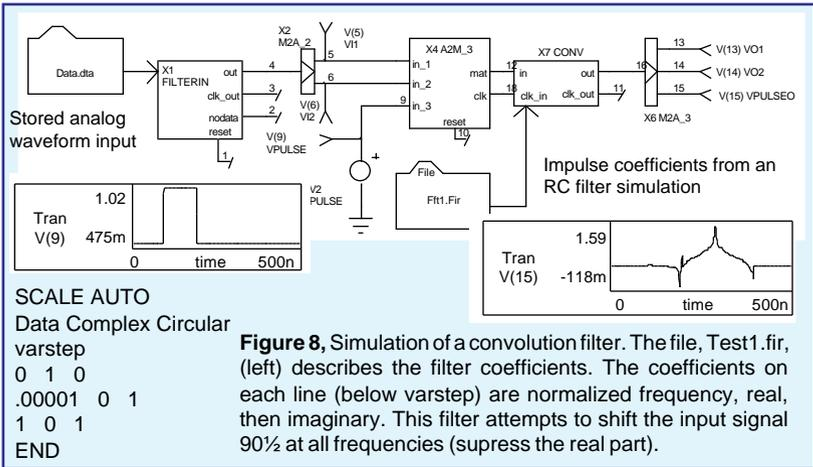
**Figure 8,** Simulation of a convolution filter. The file, Test1.fir, (left) describes the filter coefficients. The coefficients on each line (below varstep) are normalized frequency, real, then imaginary. This filter attempts to shift the input signal 90½ at all frequencies (suppress the real part).
