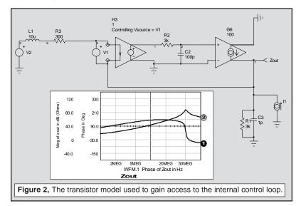
The circuit which is used to model the transistor is highly simplified when compared to the Spice model. What we want to determine from this model is whether or not external control loop cuts can provide reasonably accurate values for gain and phase margin.
