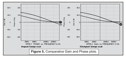
The onset of instability is predicted using the cut at the emitter and the cut at the base. Given the inaccuracy in modeling the transistor, the external loop cuts provide reasonably good results, based on classical control system theory. Finally, the original circuit stability prediction using a loop cut at the emitter (Figure 1) yields the results shown in Figure 6.
