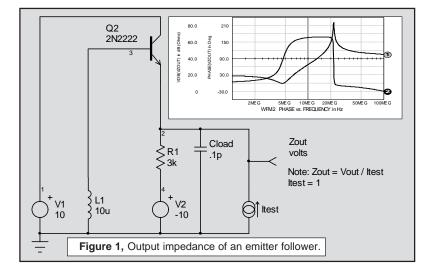
But where did the inductor come from? Base inductance can occur most commonly from long wires; for example, clip leads or test equipment wire harnesses, or from the circuit which is used to drive the emitter follower. Adding an emitter follower to an op-amp output or using Darlington connections are common circuits that add base inductance.
