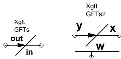
The Simulation Templates manipulate the models internally in order to configure the different simulations and access the internal node voltages and branch currents, for example  $v(xw:xgft)$  is the voltage from x to w. To accomplish this it is required that the GFT part be named Xgft.
